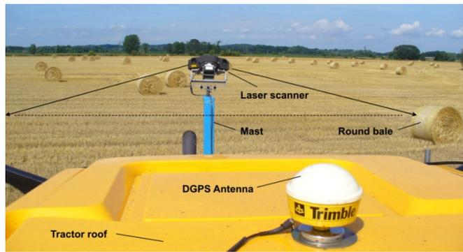
Fig. 3 Test arrangement for bale scanning
