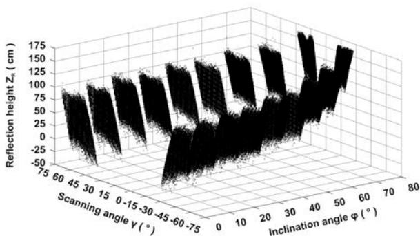
Fig. 11 Calculated height of reflection points in winter rye for different inclination angles. (Strip size: 2 x [3 m x 700 m])
