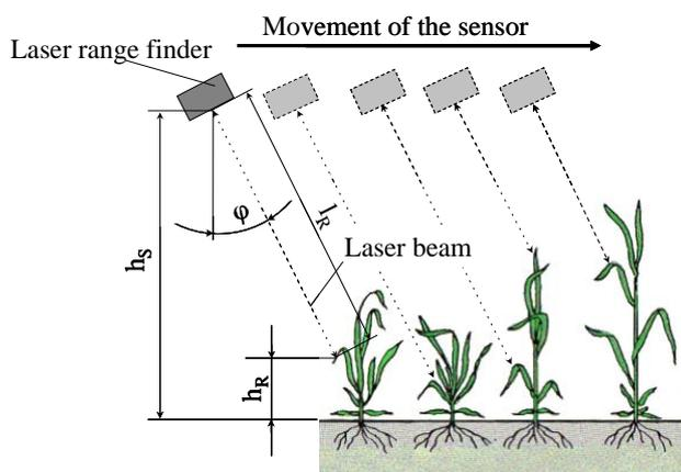
Fig. 4 Measuring principle and parameters for calculation of reflection height ( $h_R$ ).
