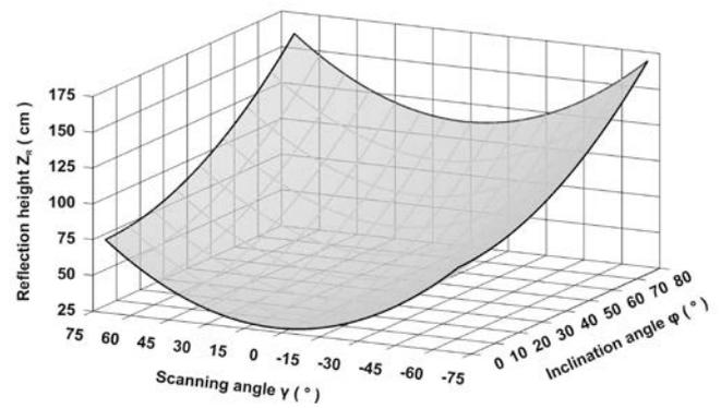
Fig. 12 Reflection height  $Z_R$  depending on inclination angle  $\varphi$  and scanning angle  $\gamma$  in winter rye.
