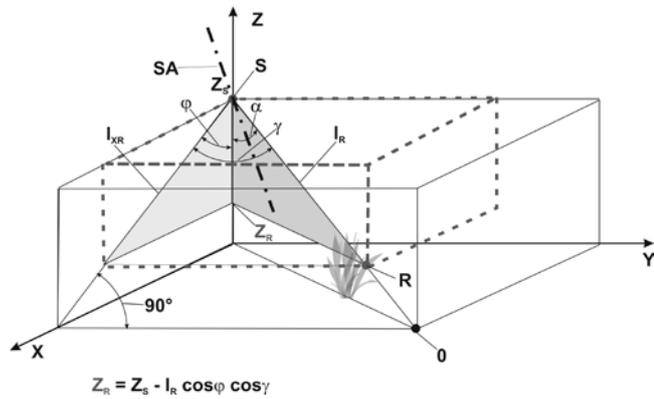
Fig. 6 Space geometry of the laser beam
