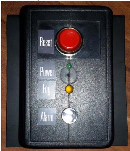
Fig.4 –Alarm module to the device FD-3
