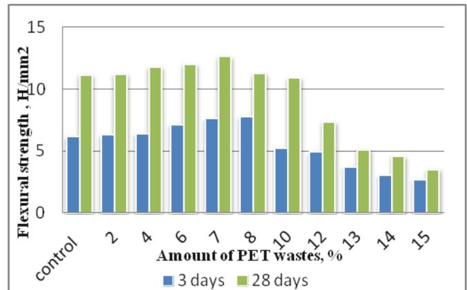
Figure 3. Results of flexural strength test for control sample and those filled with polymer wastes after 3 days and 28 days
