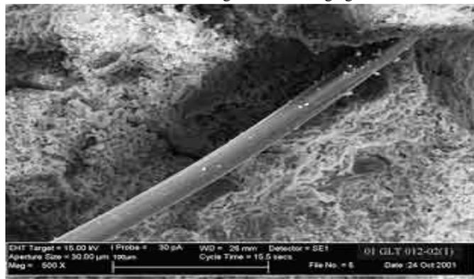
Figure 1. Lack of adhesion of cement stone with polyamide fibers. Electron micrograph [2].
