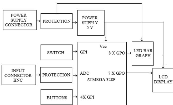
Fig. 2 Block diagram of FDI-1
