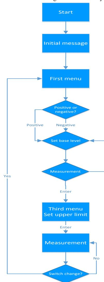
Fig. 3 Menu flow diagram of FDI-1
