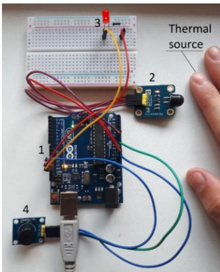
Fig 12: PIR v1.1 project assembly.
