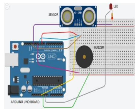
Fig. 3: Project simulation using Autodesk circuits.
