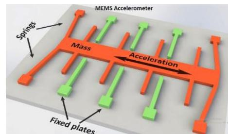
Figure 13: MEMS chip working structure and principle of action.
