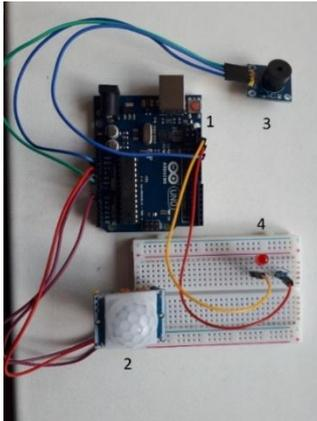
Fig. 10: PIR sensor project assembly.
