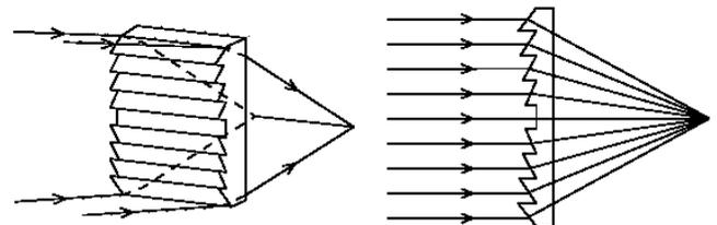
Fig.8: PIR sensor's Fresnel lens dome.
