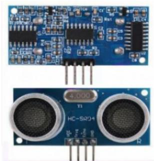
Fig. 2: HC-SR04 Ultrasonic Sensor.
