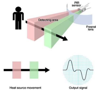
Fig. 5: PIR sensor working principle.
