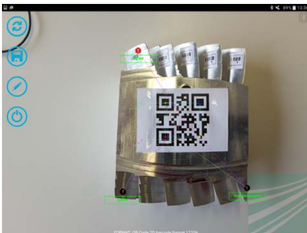
Fig. 4: Reappearance of the by verification staff with tablet marked errors on turbine blades in the display of smart glasses and other smart devices (Screen mirroring). The error markers will stay on the right place even when the smart devices move by tracking the QR code on the part.
