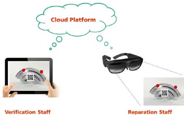
Fig. 3: Cloud-based visual inspection in quality control of turbine blade manufacturing using smart devices
