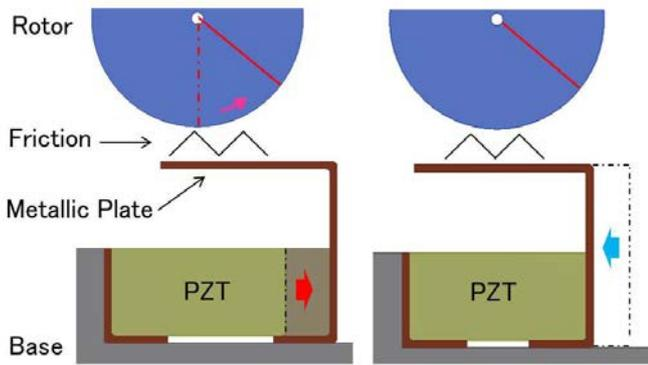
Fig. 8. Operating principle
