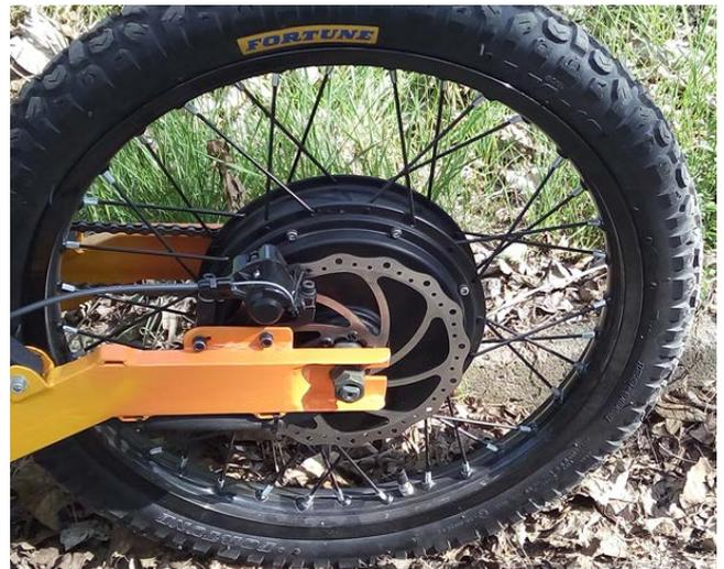
Fig. 5 Rim-integrated BLDC motor.
