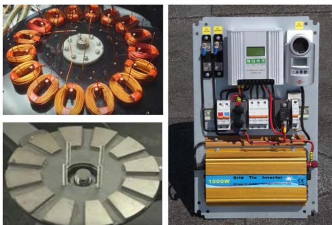
Fig. 3 BLDC motor, charge controller and grid-connected inverter.
