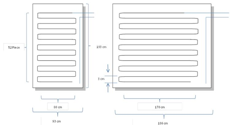
**Fig. 2** Collector dimensions
