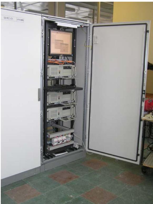
Fig. 8. Cabinet of the subsystem for processing logical dependencies of microprocessor interlocking of pointers and signals
