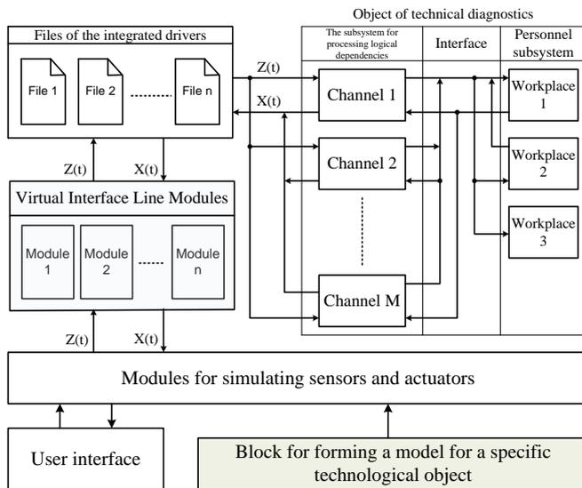
Fig. 7. The scheme for organizing a virtual interface line
