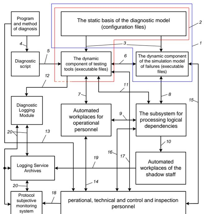
Fig. 5. Structure of intermodular interaction of components of the ergatic control system
