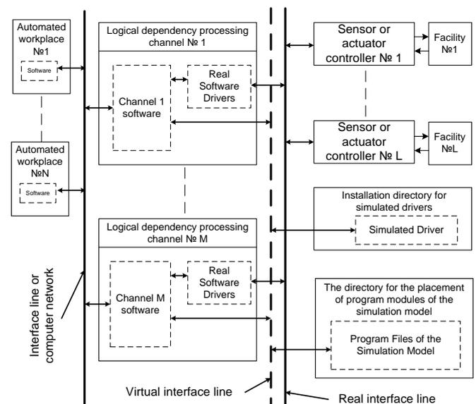
Fig. 6. Structural-functional diagram of the automated control system in conditions of interactive interaction with personnel
