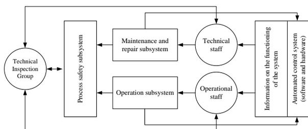
Fig.1. The existing scheme for ensuring the safety of automated control systems
