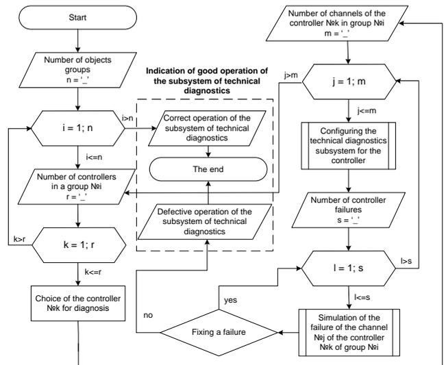
Fig. 4. Algorithm of periodic monitoring of the subsystem of technical diagnostics
