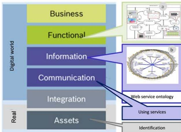
Fig.7: IT structure of quality operations management system based on RAMI 4.0
