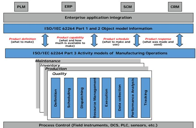
Fig.2: ISO/IEC 62264 Manufacturing Architecture [9]
