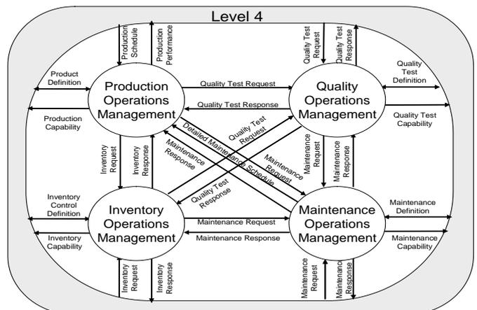
Fig.3: Interrelations between the areas of manufacturing operations management [7]
