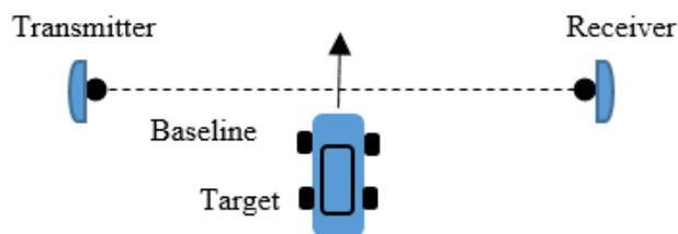
**Fig. 1:** Illustration of acoustic forward scattering configuration.
