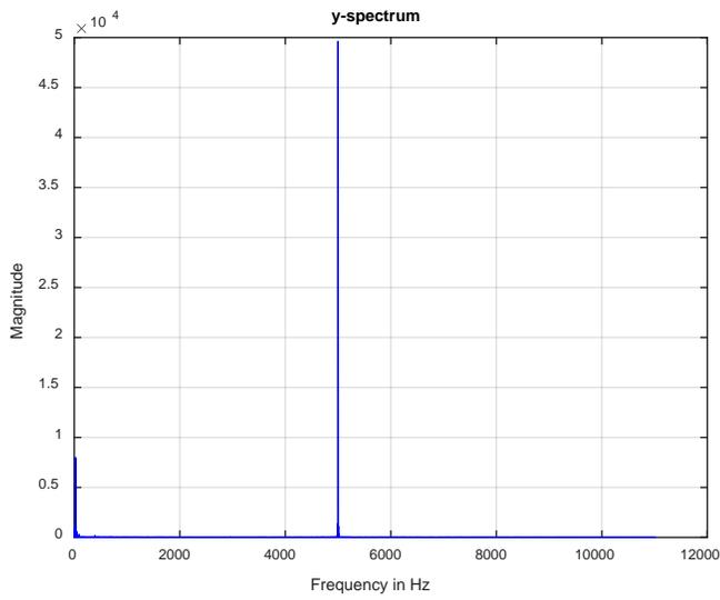
Fig. 7: Spectrum of the recorded sound signal.
