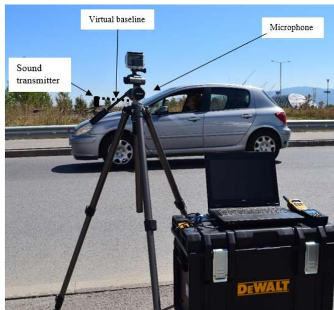
Fig. 4: Sound recording system.
