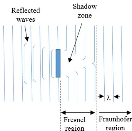
**Fig. 2:** Sound diffraction.
