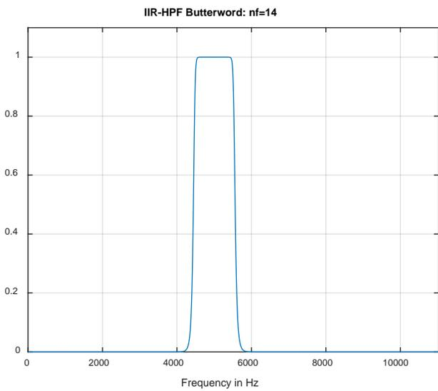
Fig. 8: Frequency response of the bandpass filter.
