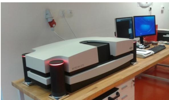
Fig. 2 Microtomographic device SkyScan 1272 including the workstation
