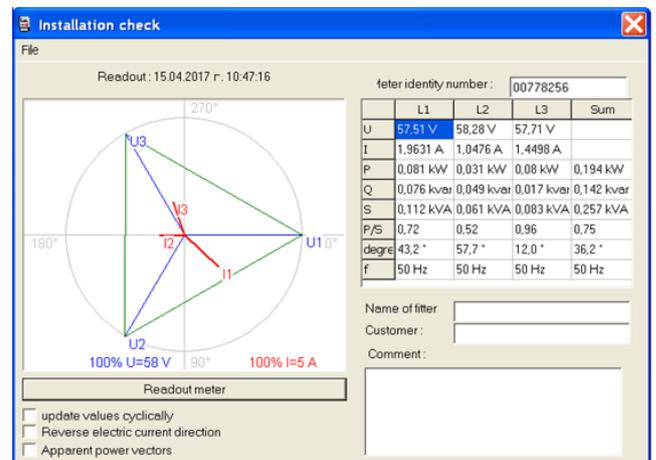
Fig.3. An unbalanced induction furnace with a network frequency.
