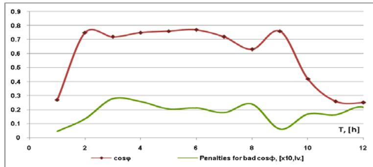
Fig. 7. Modification of power factor in basic mode and finishing with 'marsh' 40% and penalties for bad cosφ.
