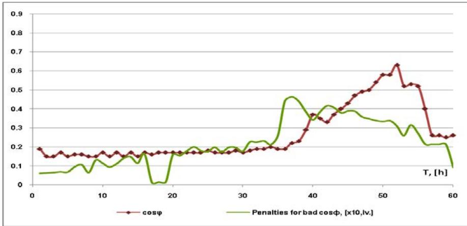
Fig. 5. Modification of power factor in sintering mode and penalties for bad cosφ.
