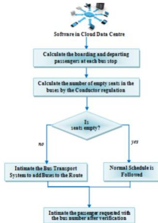
Fig.4. Function of software in cloud data center [3]
