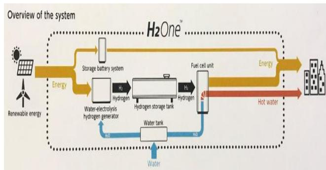
Fig. 5 Overview of Toshiba H<sub>2</sub>One™ system.
