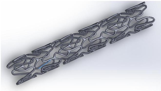
Fig. 9. 3D model of the ISMA stent
