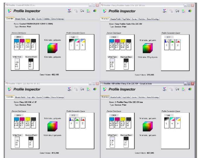
Fig.5 - Comparison of the basic parameters of the studied color profiles (factory-bottom left; iProfiler - bottom right; Fiery Color Profiler - top right) versus standard offset profile Fogra 39 (top left)
