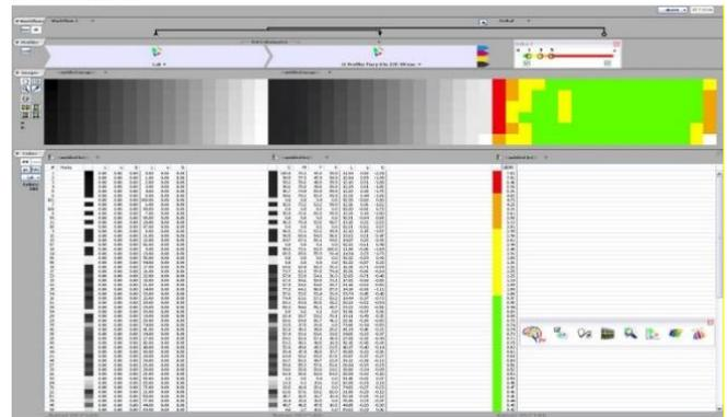
**Fig.7 - Neutral color rendering evaluation through generated individualized profile with i1Profiler software**
