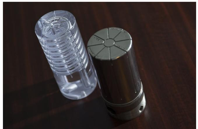
**Fig. 3.2** A Bastech mold core insert with conformal cooling channels prototyped using 3D Systems' Stereolithography (SLA) technology and printed in maraging steel on the ProX® DMP 200. (Source: 3dsystems.com)
