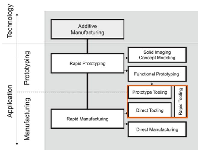
Fig. 1.1 AM: rapid tooling, defined as a subcategory that integrates prototype tooling and direct tooling (Source: [4])
