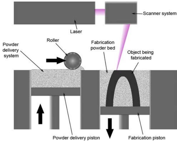
**Fig.2.1** Selective Laser Melting (SLM) – Schematic
