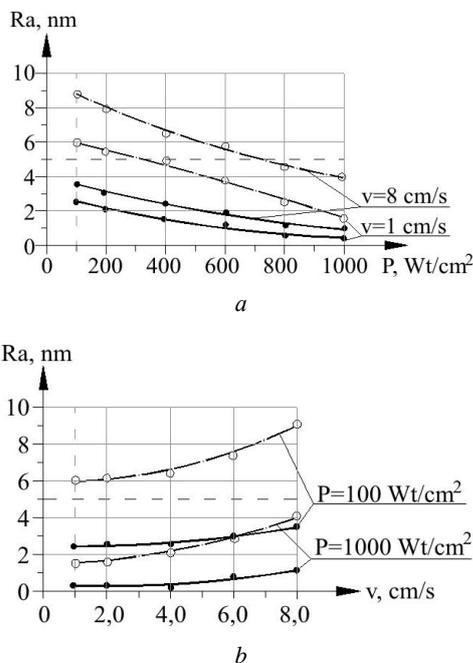
Fig. 4. Dependence of the average arithmetic roughness of the nanorelief Ra on the specific power of the electron beam  $P_{\text{ннт}}$  (a) and the speed of electron-beam micromachining  $V_{\text{ннт}}$  (b):  $\circ$  – by the works [8, 9];  $\bullet$  – by
