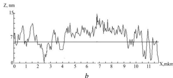
Fig. 2. Appearance (a) and nanorelief along the AB (b) line of the surface area ( $12 \times 12 \mu\text{m}$ ) of the fragment of the plate of the optoelectronic capacitance sensor from K8 glass with a metallic thin silver film fused in its surface by an electron beam (film thickness 350 nm).
