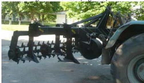
Figure 3 – Garden chisel plow with roller
