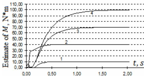
Fig.4 - Transition processes of identification of the external moment of load
