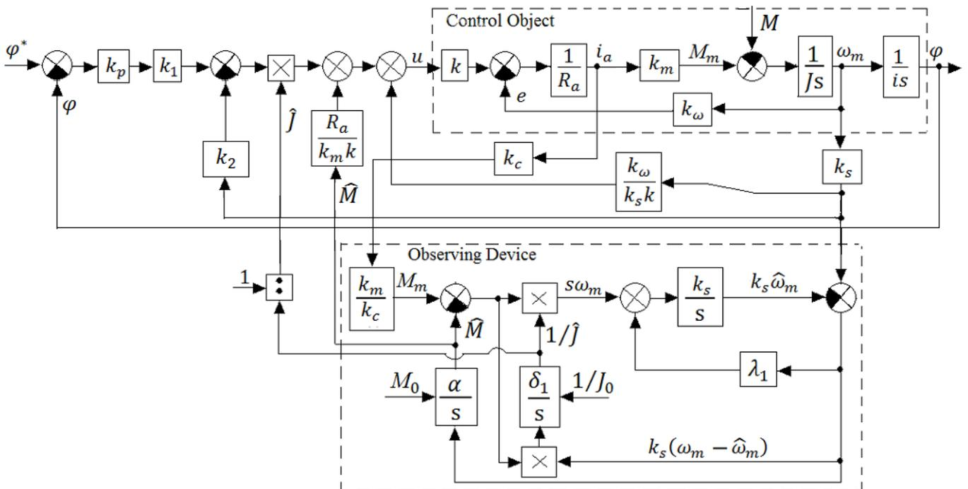
Fig.1 - Block diagram of the load adaptive system of automatic control of drive
