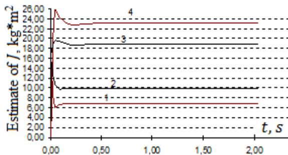
Fig.3 - Transition processes of identification of the moment of inertia of load
