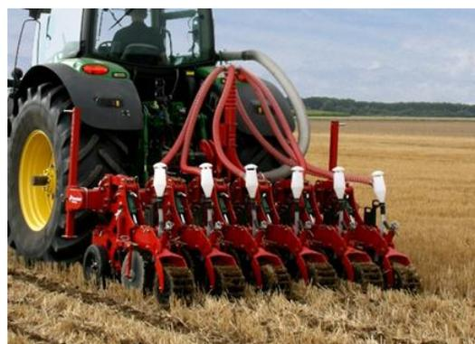
*Fig.6. Strip tiller with central dosage*
