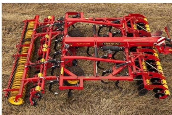
*Fig.3. Chisel cultivator with disk-type cutting section*
