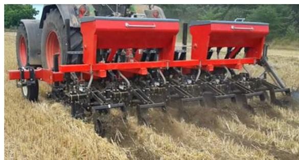
*Fig.5. Strip tiller with individual fertiliser dosage*
