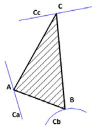
Fig 2.: Paths of points A and C are straight lines, and path of point B is circle
