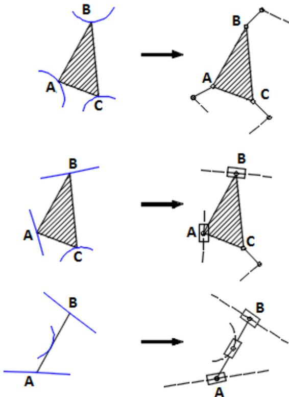
Fig 7. : Transformation of geometric problems into mechanisms
