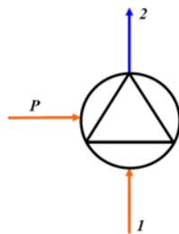
Fig. 1. Sea water pump symbol with marked inlets (inputs) and outlet (output)
