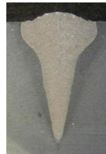
Fig. 1 Weld cross-section, obtained at: L = 6 mm, F = 3 kHz, \gamma = 0 , v = 5 mm/s, I_b = 55 mA.
