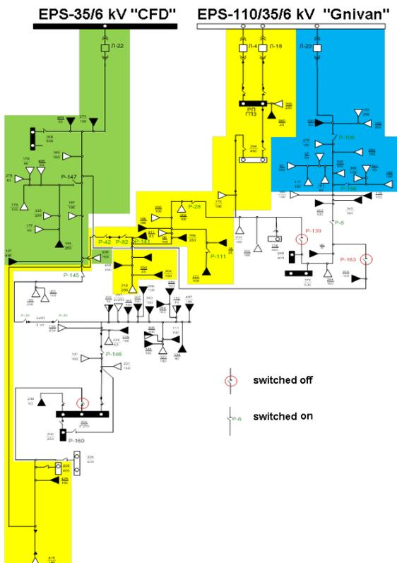
Fig. 2. The branch circuit with figured out unconditional attractor feeders and a boundary zone
