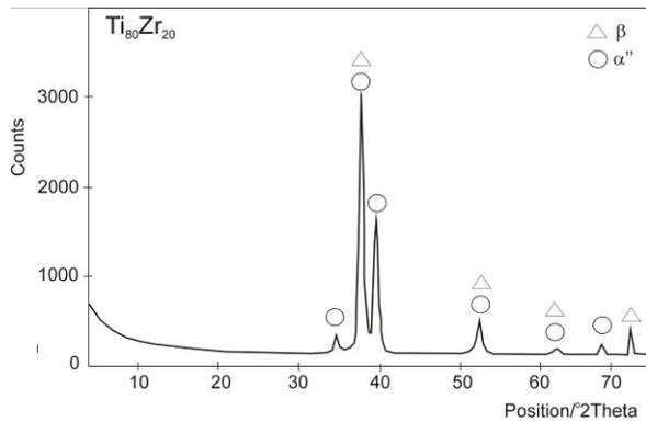
Fig. 1b XRD analysis of alloy containing 20 at.% Zr
