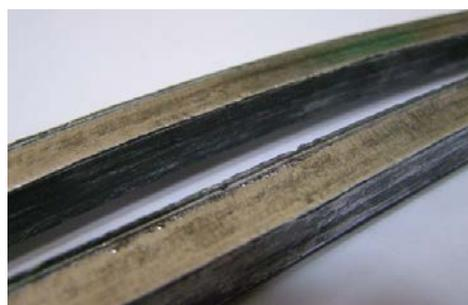
Fig. 2. CP Ti samples after SPD processing
