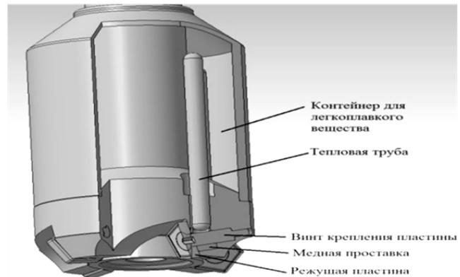
Fig.2 –Combined mill with integrated cooling system
