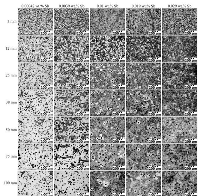
**Fig. 2** Optical micrographs of the central part of the wall thicknesses of 3, 12, 25, 38, 50, 75 and 100 mm at various Sb contents (etched in Nital).
