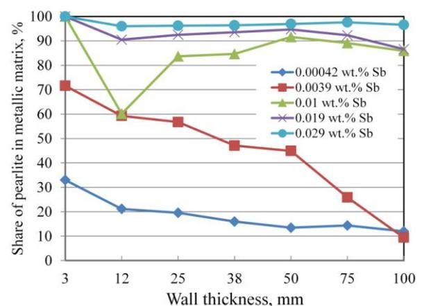
**Fig. 3** Effect of Sb addition on the share of pearlite in the metallic matrix of the wall thickness of 3, 12, 25, 38, 50, 75 and 100 mm.
