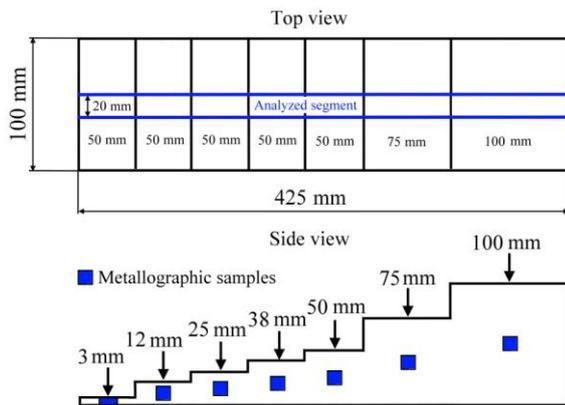
**Fig. 1** Schematic show of the step wedge test blocks and places where samples for metallographic analysis were taken.
