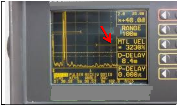
Fig.2. Display of calibration parameters for UT of castings
