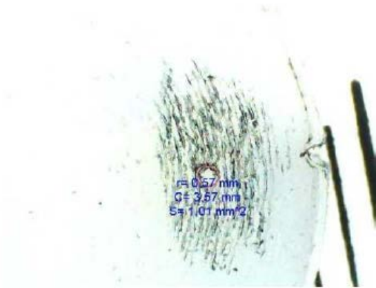
Fig. 6 Example trace of wear on the flat surface, r_o=0,258 mm, S=0,209 mm 2 .
