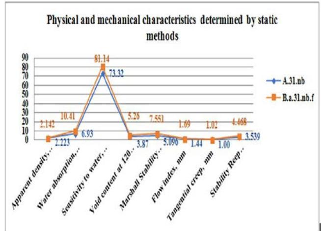
**Fig. 5 –** The values of physical - mechanical characteristics determined by static methods
