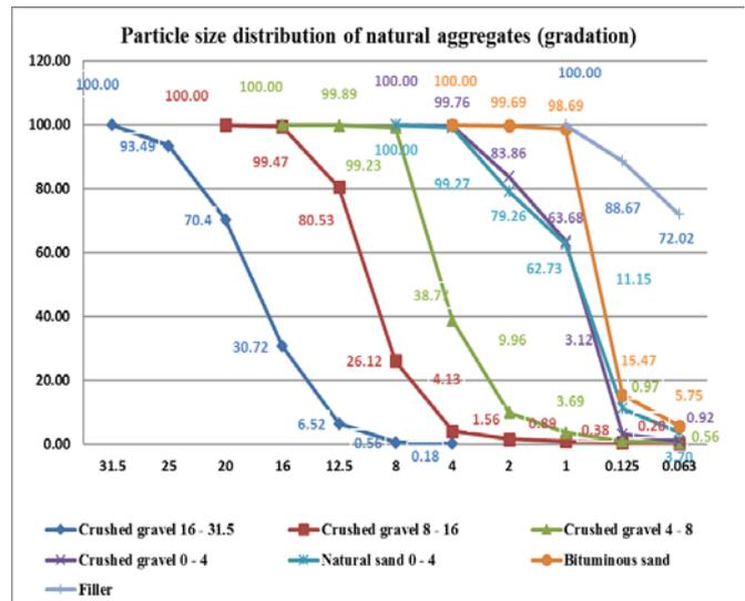
Fig. 3 – Particle size distribution of natural aggregates (gradation)
