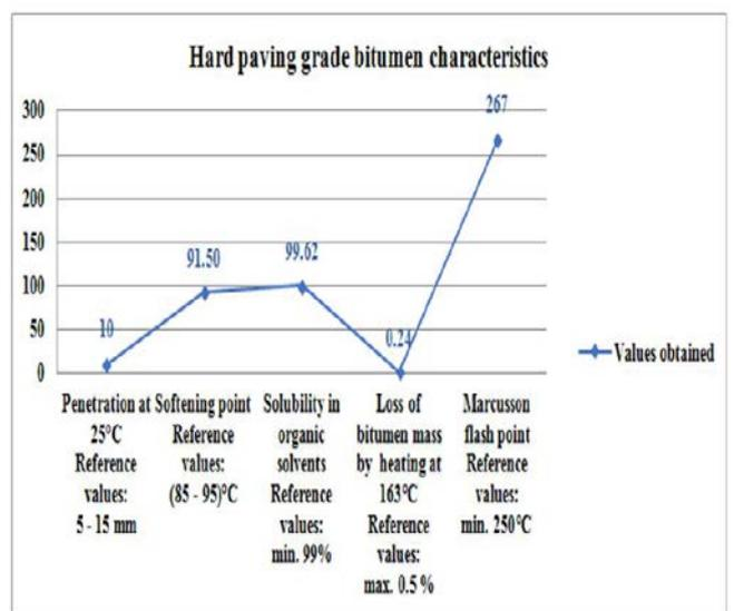
Fig. 4 – Hard paving grade bitumen characteristics
