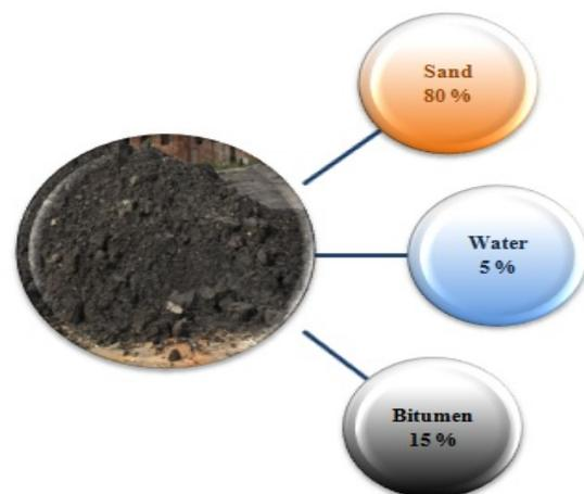
Fig. 1 Bituminous sand composition (Dayna Linley, 2010).
