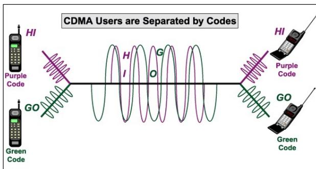
A binary signature sequence (codeword) is assigned to each user in a CDMA system. The data to be sent is mapped onto the codewords and the different users codewords are mixed together and sent over the channel. At the receiver end a decoder, which is individual for each user, compares the incoming sequence with stored copies of the codewords to be able to extract the information bits.
