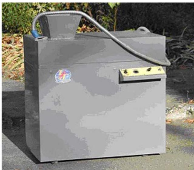
**Fig. 7.** Experimental unit for the preparation and application of a graphite-aqueous suspension
