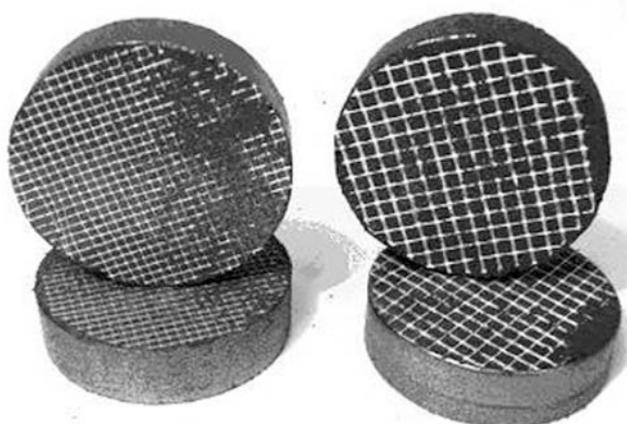
**Fig. 6.** Extruded sorption elements, reinforced by polymer mesh
