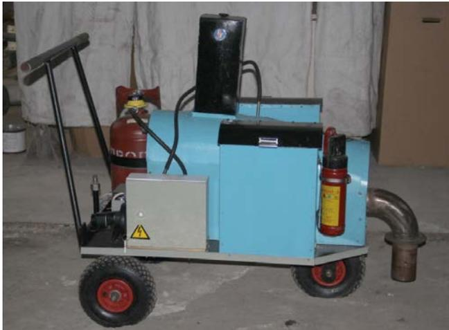
**Fig. 2.** Autonomous automatic aggregate of a local destination with capacity of 1-2 m<sup>3</sup>/h by TEG
