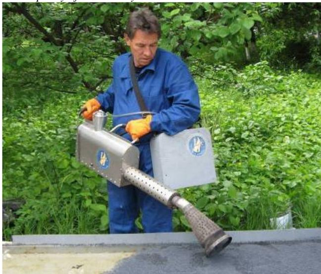
**Fig. 3.** TEG autonomous knapsack generator with a capacity of 0.8 m<sup>3</sup>/h (3 kg/h by raw material).
