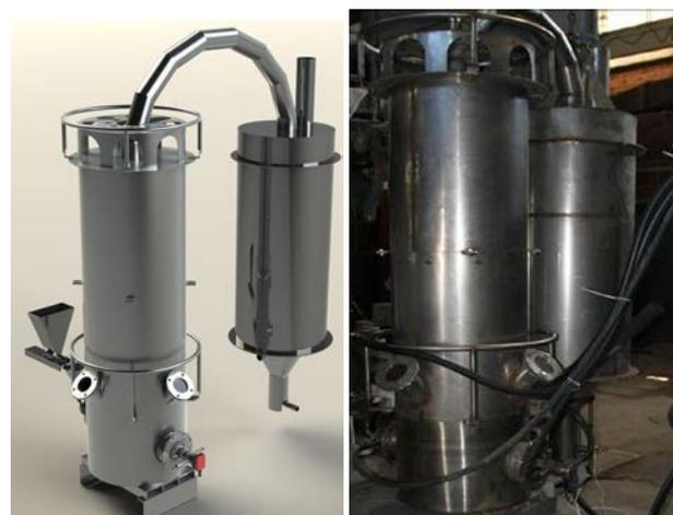
**Fig. 1.** Pilot unit for TEG generation with a capacity of 8.5 m<sup>3</sup>/h Simulation (left). In metal (right)
