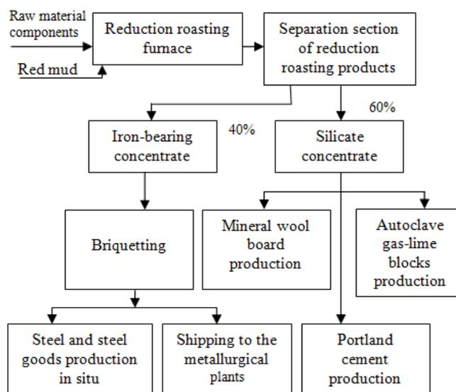
**Fig.** The general technological scheme of pyrometallurgical conversion
