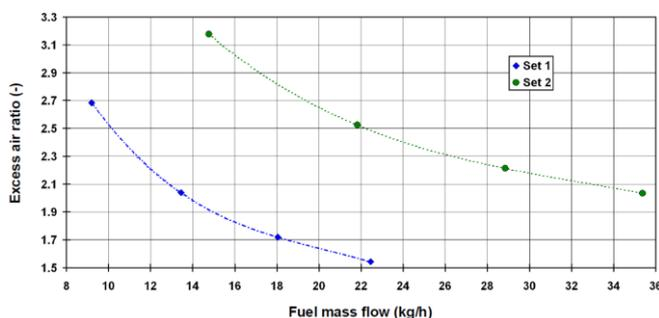
Fig. 4. Engine excess air ratio change for each measurement set
