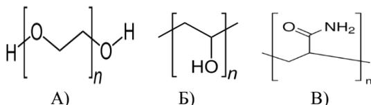
Fig.2 Artificial water-soluble polymers: A) polyethylene glycol; B) polyvinyl alcohol; C) polyacrylamide
