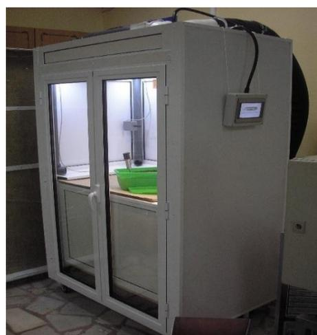
Fig.11. Chamber with controllable parameters of heat, light and humidity of soil and air
