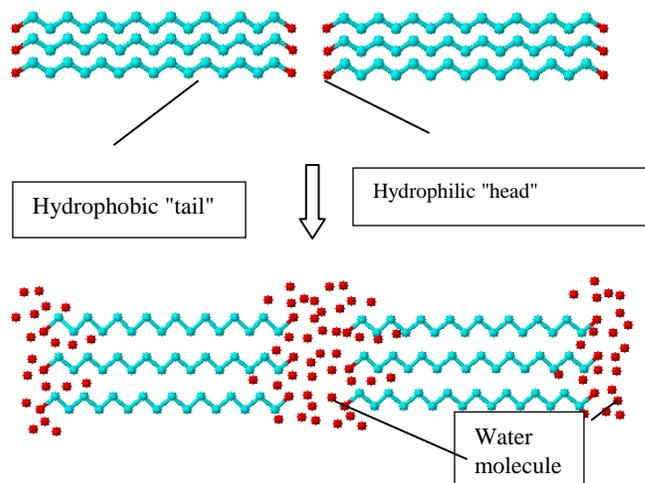
Fig.3. Molecule structure of water-soluble polymers and mechanism of water molecule diffusion through them
