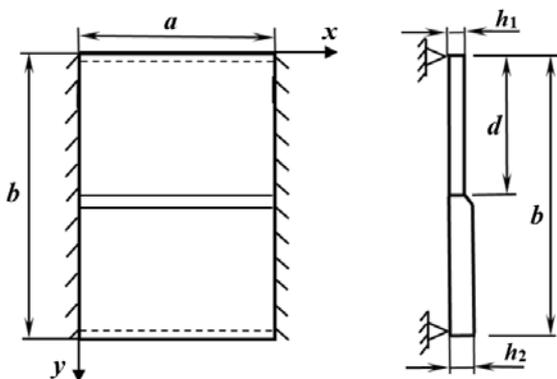
**Fig. 2.** Rectangular plate with variable thicknesses.
