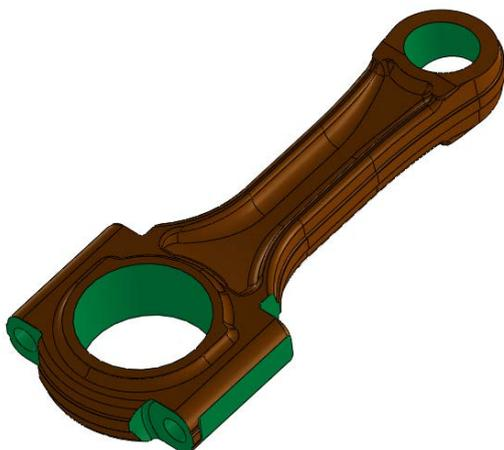
Fig.9 : Optimized connecting rod
