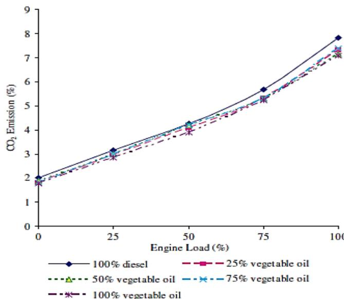
Fig. 6 Comparison of CO<sub>2</sub> emission versus engine power output for different fuels/oil blends [4].
