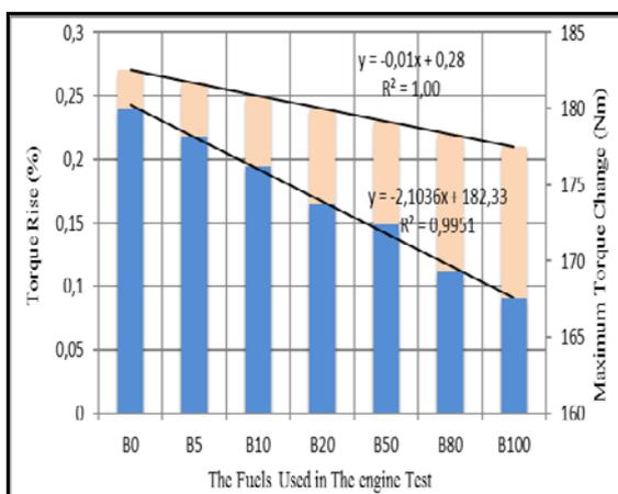
Figure 4. Change in the torque rise and maximum torque curves based on the fuels used
