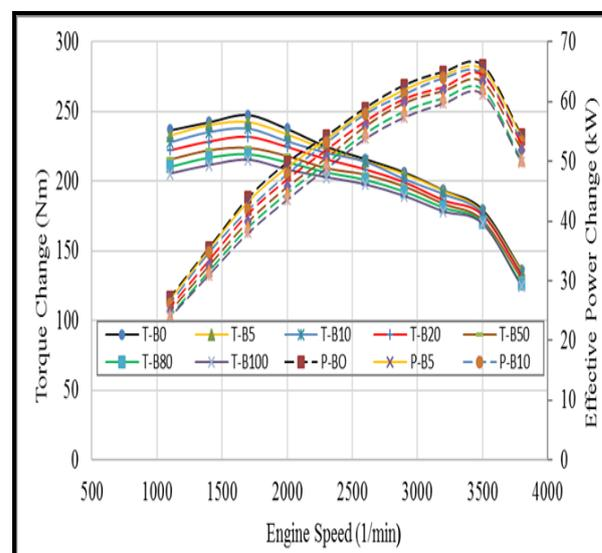
Figure 2. Changes in maximum torque and torque at the nominal speed
