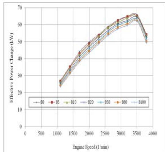
Figure 1. Effective power changes in diesel (B0) fuel and diesel-biodiesel mixtures based on engine speeds
