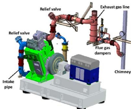
Fig. 2 Single cylinder research engine (SCE).
