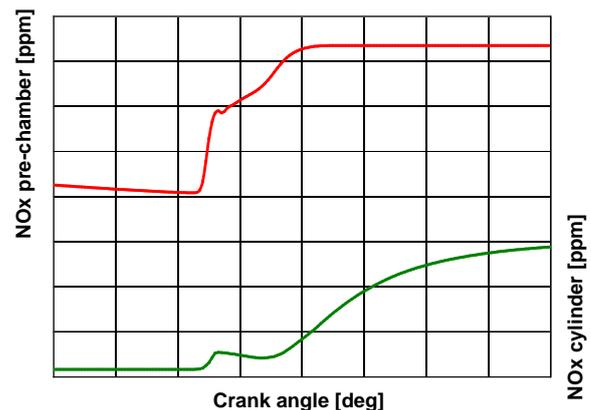
Fig. 5 Simulated NO<sub>x</sub> concentrations with the NO<sub>x</sub> submodel in the prechamber and in the cylinder of a large gas engine.
