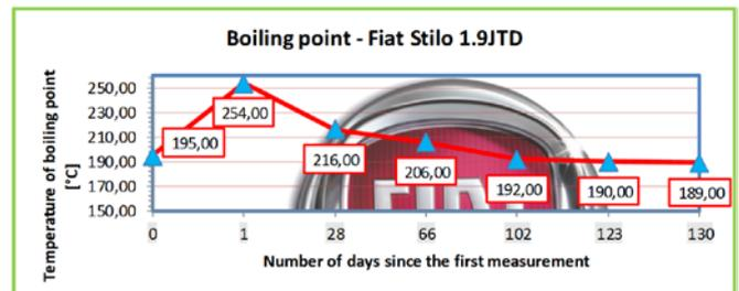
Fig. 4 Decline in boiling point of brake fluid in terms of operation time (after refilling by new brake fluid).
