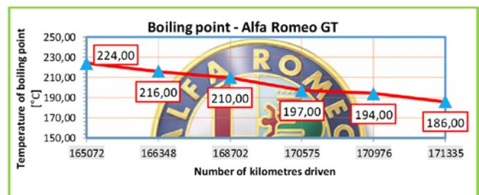
Fig. 3 Decline in boiling point of brake fluid in terms of driving performance.
