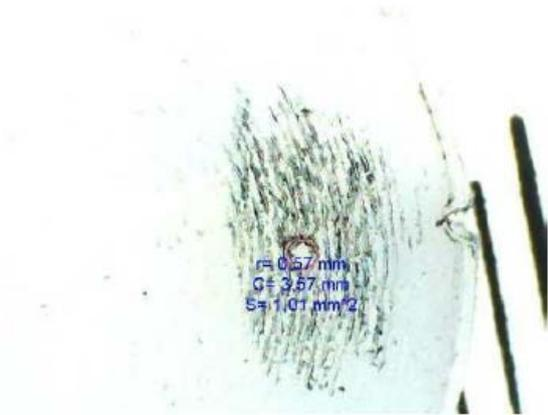
Fig. 6 Example trace of wear on the flat surface,  $r_o=0,258$  mm,  $S=0,209$  mm<sup>2</sup>.
