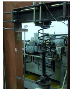
Fig. 1. Spring characteristic test bench.
