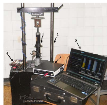
Fig. 3. Shock absorbers tester.
