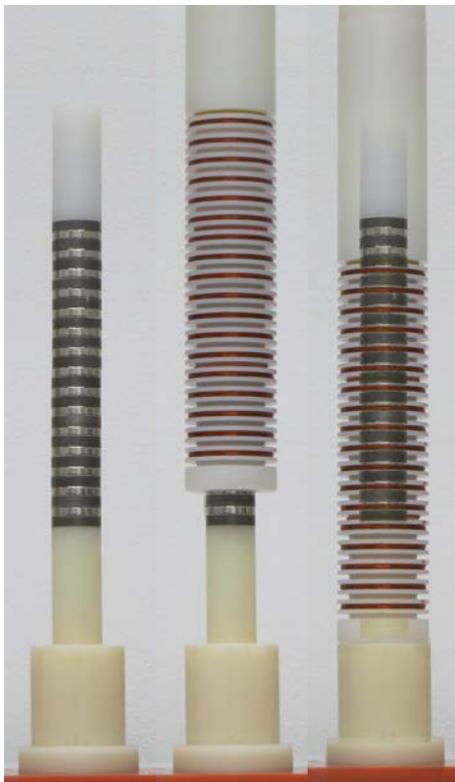
**Fig. 3** Experimental prototype of electromagnetic vibrating generator. From the left hand side is the „backbone“ consisting from FeNdB permanent magnets and soft ferromagnetic spacers. The improved coil assembly consisting of holder with copper coils during the vibration motion (upward and downward).
