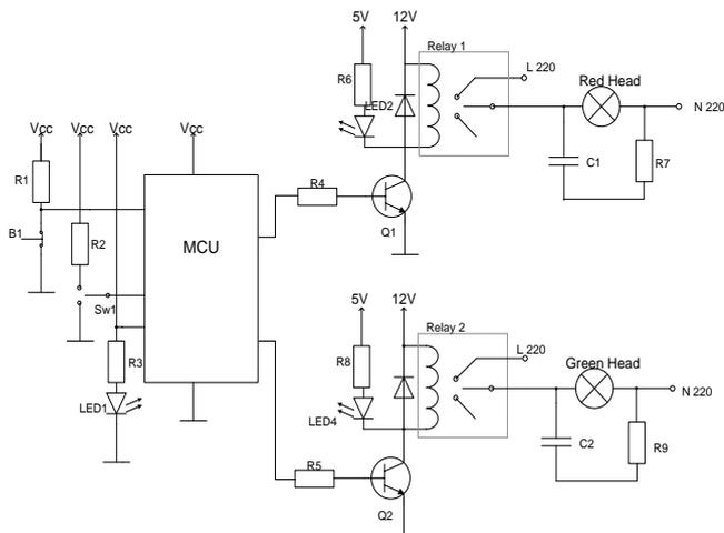
Fig. 2 Controller for simulating traffic light sequences.
