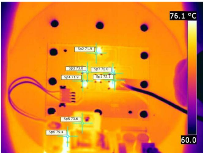
Fig. 5. First Green LED head at 81s on time 39s off
