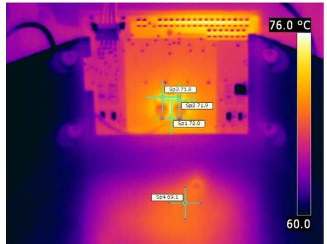
Fig. 9. Second Green head at 81s on 39s off time
