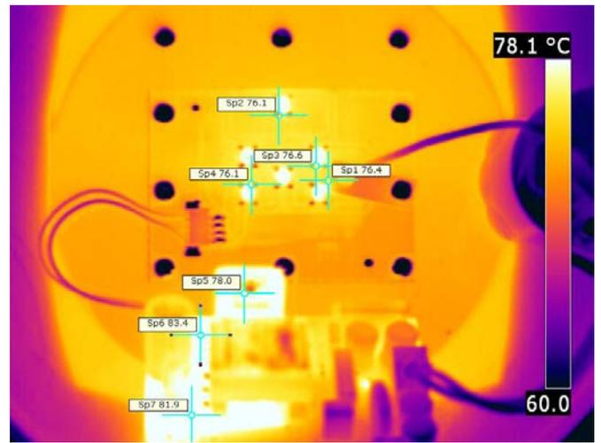
Fig. 8. First Red head at constant on mode
