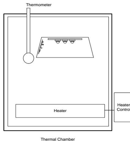
Fig 3 Tested signal head in thermal chamber.
