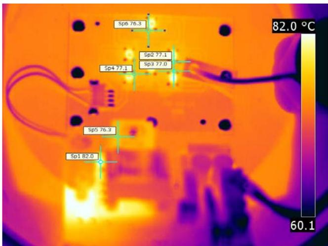
Fig. 6. First Green LED head at constant on mode
