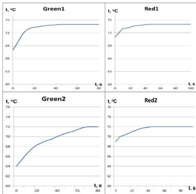
Fig. 4 The rise of temperature over time for each of the examined LED heads
