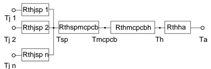
**Fig. 1** Thermal resistance model of multiple LED chips on common MCPCB attached to heatsink.
