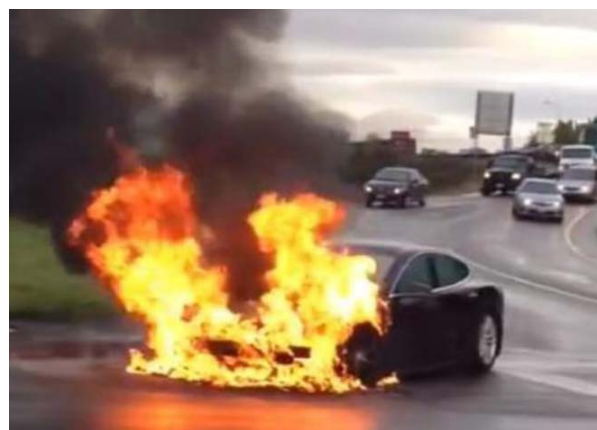
Fig. 3 Tesla S vehicle on fire due to penetration of the batteries and causing a short circuit [6]
