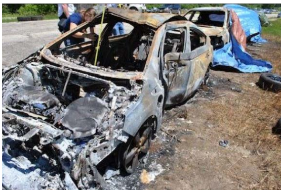
Fig. 2 Chevrolet Volt car that caught fire in the garage [6]
